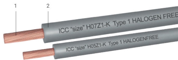
1. Rame flessibile Classe 5 CEI EN 60228 | Flexible copper Class 5 CEI EN 60228 2. Mescola termoplastica T17 LSOH | Thermoplastic compound T17 LSOH
