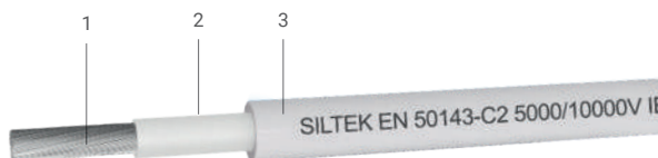
1. Rame flessibile Classe 5 CEI EN 60228 | Flexible copper Class 5 CEI EN 60228 • 2. Gomma siliconica EI2 | Silicone rubber EI2 • 3. Tipo D2 Mescola zero alogeni | Type c2 Halogen free compound
