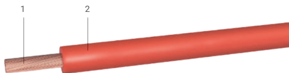
1. Rame rosso flessibile Cu-ETP1 (JASO D 609-90) | Flexible bare copper Cu-ETP1 (JASO D 609-90) • 2. PVC (polivinilcloruro) esente piombo | Lead free PVC (polyvinylchloride)
