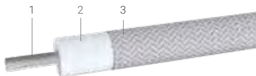
1 – Rame flessibile / Flexible copper 2 – Gomma siliconica / Silicone rubber 3 – Treccia in fibra di vetro / Fiber-glass braid
